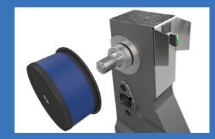
The new quick clamping system for chucks enables tool-free replacement in a matter of seconds.
