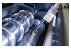
**Positioning aid** Time-saving and precise alignment for bottom knife and razor blade grooved bushes.
