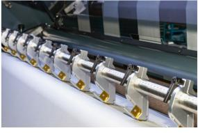
Razor blade cut Reasonable and good. Optionally as groove or mirror cut.
