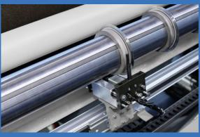
**Automatic knife positioning** For repeating exact slitting positions and set-up time reduction.
