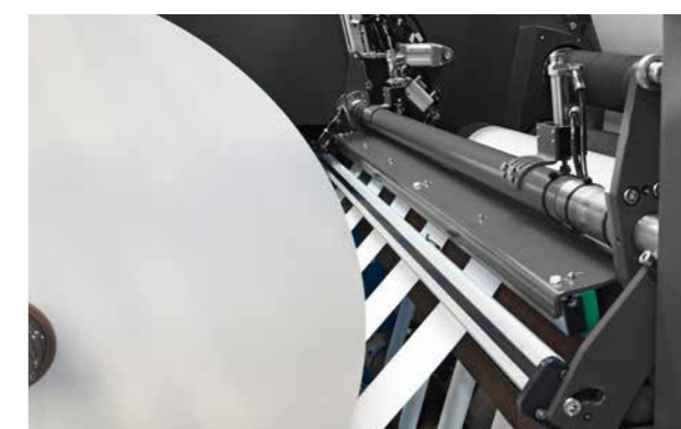
Cross cutting Automatic cross cutting and lay-on for fast roll change.
