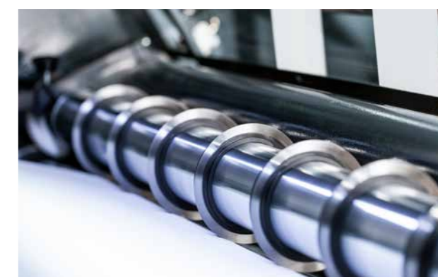
Scissor shear cut For best quality with long service life. Optionally with automatic positioning and single knife holders.
