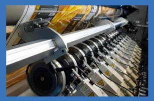
Scissor shear cut / razor blade cut Optionally in combination with single knife holders.
