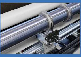
**Automatic knife positioning** For repeating exact slitting positions and set-up time reduction.
