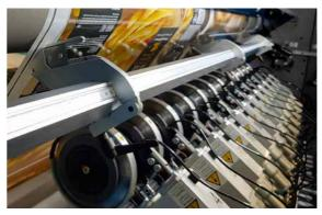
Scissor shear cut / razor blade cut
